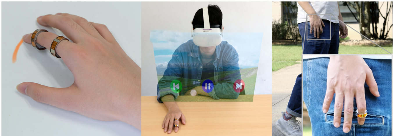
Figure 1: Left: MouseRing is an IMU ring-shaped device that facilitates continuous on-surface finger tracking. Middle: MouseRing is an always-available pointing technique in VR, AR, large-screen interactions, etc. Right: MouseRing supports both single-ring and dual-ring interaction on diverse surfaces.
